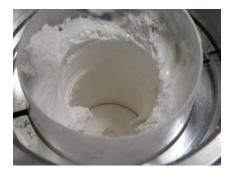
**Figure 7.** Aborted experiment trying to disperse 27 vol.-% of BN in UP-resin. All material clogs to the wall while the dissolver blade (not shown) is mixing only air.
